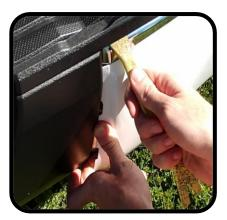
6. Slip the inboard edge under the plastic center cover. Slide the cover upward until it is completely tucked under the step pad and center trim. Be careful not to let the tape firmly attach until you are completely satisfied with the position of the cover.
